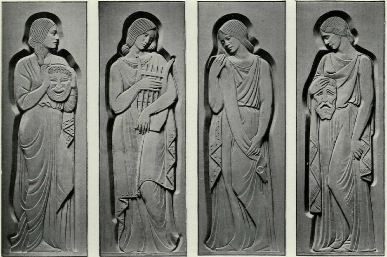
PLASTER CASTS OF THE SCULPTURE FROM WHICH REVERSE MOLDS WERE MADE THE REVERSE MOLDS WERE ASSEMBLED IN THE FORMS ON THE BUILDING AND THE CONCRETE CAST INTEGRAL WITH THE STRUCTURE
