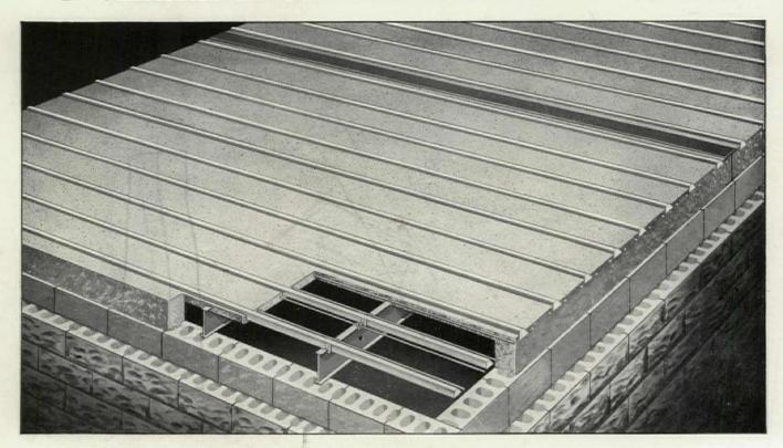
There can be no shrinkage of floor joists with the J & L Steel and Concrete Floor System. It forms a rigid, vibrationless base for framing of any material. It eliminates troublesome and costly repairs necessitated by the shrinkage that occurs invariably when wooden floor joists are used. It is also fireresistant and vermin-proof.
