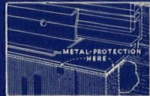
A sturdy square-cut continuous metal flange projects over edge of facing material, shielding the area which is most vulnerable.
