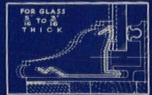
Glass-holding units and face members are self-adjusting to various glass thicknesses without tilting inward or outward.
