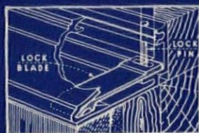
A metal blade inserted in each end of face and locked by pin in rear member is an extra means of securing face in position.
