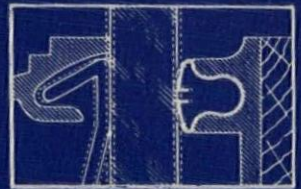
The metal surfaces which contact the sides of glass act as a yielding cushion, absorbing dangerous shocks and jars.
