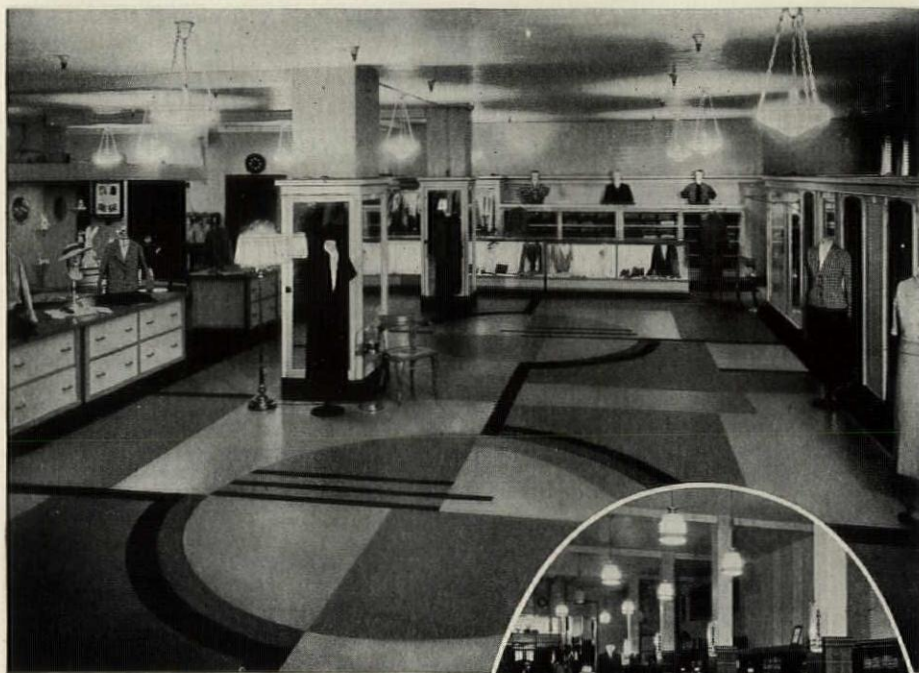
ABOVE—This custom-cut Armstrong's Linoleum Floor in sportswear department of Elder and Johnston Company, Dayton, is Armstrong's Plain Linoleum in ruby, black, orange, jade, and tan. Armstrong's Architects' Service Bureau offers, without charge, complete technical assistance in the design of modern floors.
