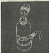
Ideal Variport Valve—regulates venting rate on 1 pipe steam or
