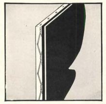
While in a molten state during the manufacturing process, these three sheets of glass are fused into one homogeneous unit.
