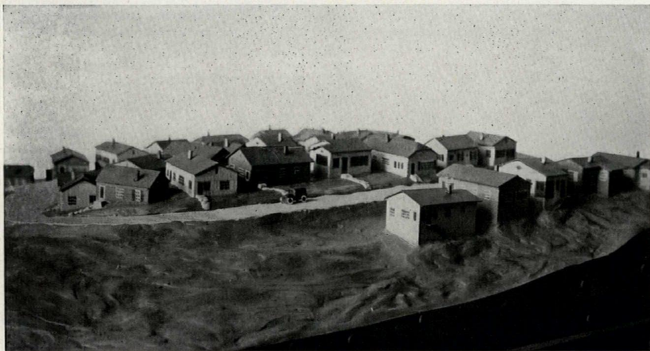
In studying the arrangement of a group of miners' cottages proposed at Inspiration, Arizona, the architects, Johnson, Kaufmann & Coate, enlisted the services of McCallum to make this model which accurately depicts the site. Four types of cottages—with variety obtained through several colors for walls, roofs and shutters—were used and each cottage was modelled as a unit. All were first assembled on a field of sand
