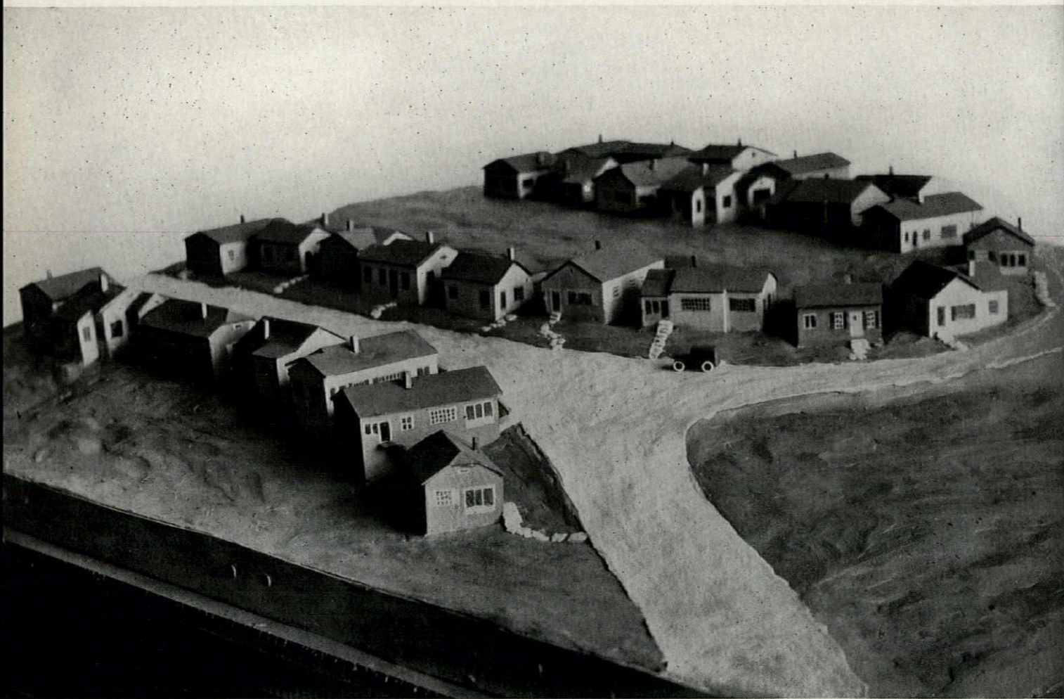
In studying the arrangement of a group of miners' cottages proposed at Inspiration, Arizona, the architects, Johnson, Kaufmann & Coate, enlisted the services of McCallum to make this model which accurately depicts the site. Four types of cottages—with variety obtained through several colors for walls, roofs and shutters—were used and each cottage was modelled as a unit. All were first assembled on a field of sand
