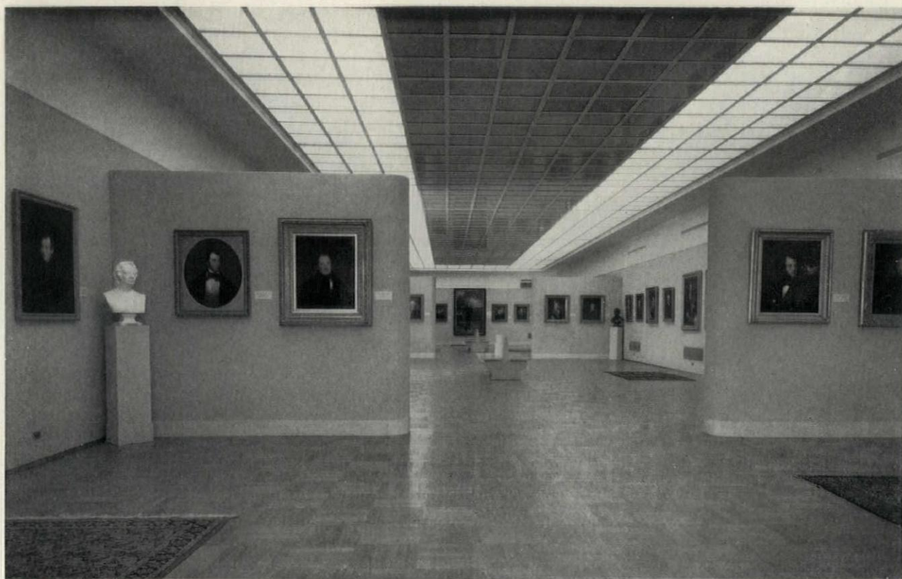
The great upper galleries of the New York Historical Society, above, are top-lighted with the central area of the light darkened to eliminate glare on the polished floor and intensify the illumination of paintings on all the walls
