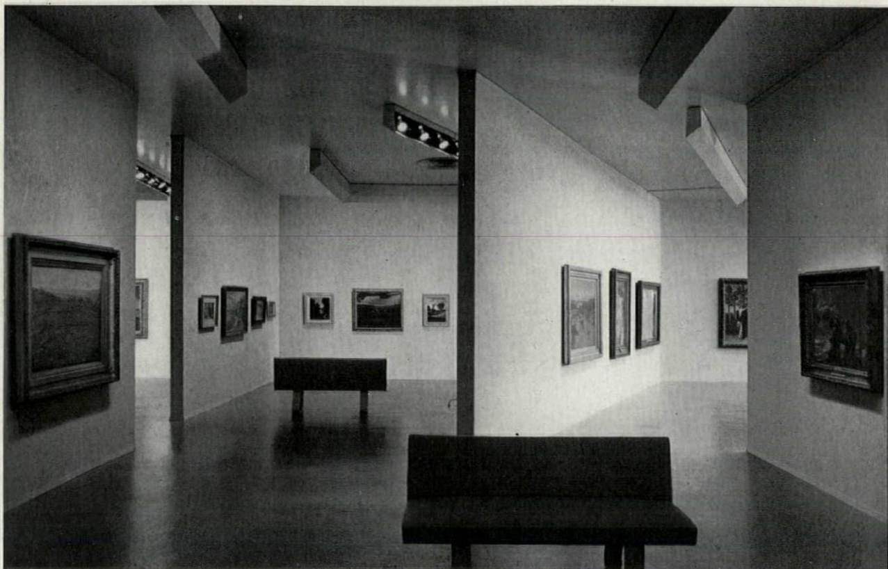
Gallery partitions, lighting fixtures, and even asbestos panels used to modulate light from the translucent south wall, all can be arranged at will to accommodate the changing exhibitions. The photos on these pages by Damora
