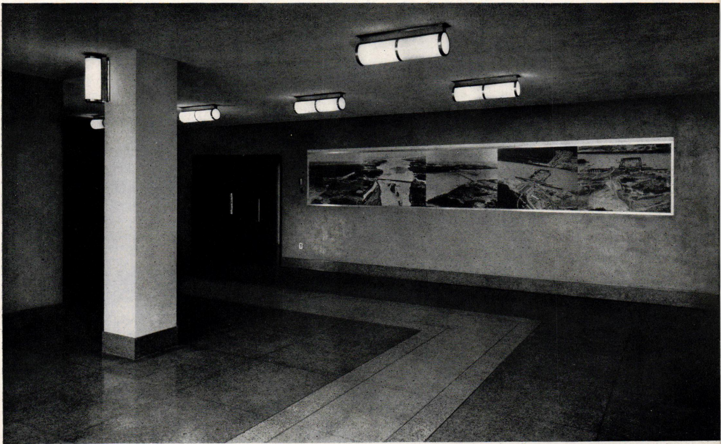
LOBBY ON LOWER FLOOR OF WHEELER, WHERE VISITORS REENTER BUILDING AFTER TOUR OF PLANT. LIGHT FIXTURES CONTAIN FIVE BULBS WITH FILA- MENTS CENTERED IN CYLINDERS. FLOOR AND BASE, LIGHT GRAY TERRAZZO. PATH TO ELEVATOR, WHITE WITH YELLOW EDGE. CEILING, CANARY YELLOW
