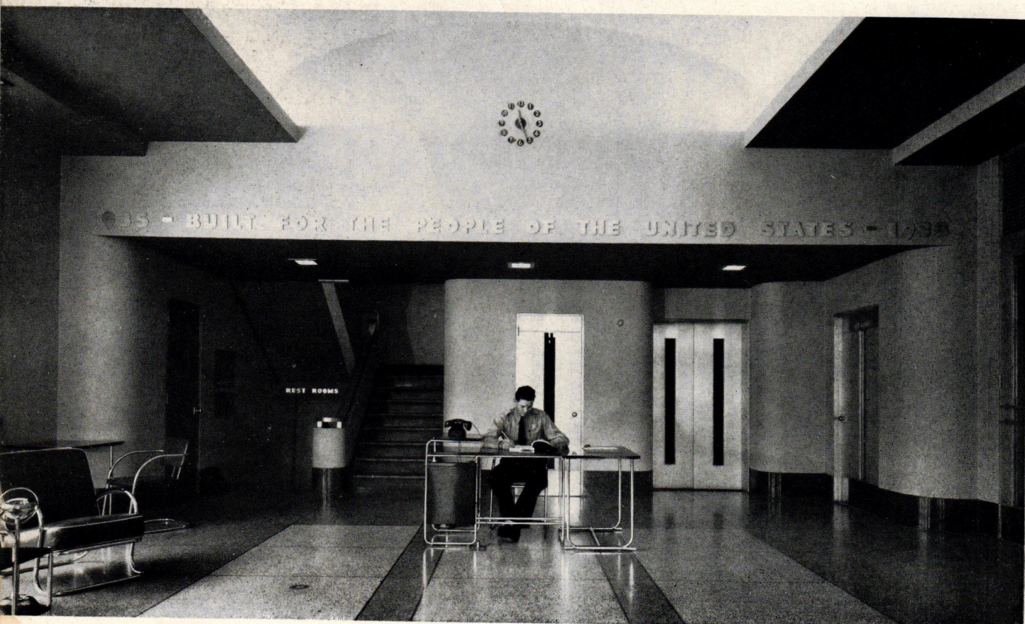
NORTH VIEW OF PICKWICK POWERHOUSE TAKEN FROM TOP OF DAM. BELOW IS RECEPTION LOBBY AS SEEN FROM INSIDE ENTRANCE DOORS. REDDISH BROWN AND WHITE TERRAZZO FLOORS WITH RED-BROWN BASE AND BURLAP-COVERED WALLS PAINTED GRAY ARE BRIGHTENED BY BLUE SOFFITS AND LEMON YELLOW PLASTER CEILING. ALUMINUM FURNITURE, UPHOLSTERED BLUE, AND ALUMINUM DOORS FURNISH SHARPER ACCENTS IN THIS ORDERLY ENSEMBLE
