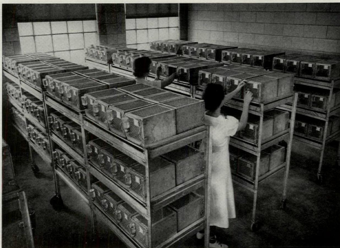
THE TOP ILLUSTRATION SHOWS A TYPICAL LABORATORY. NOTE THE FLUSH LIGHTING FIXTURES AND THE SURFACE TYPE SPRINKLER HEADS. THE LOWER PHOTOGRAPH SHOWS A TYPICAL CAGE ROOM IN WHICH TEST ANIMALS ARE HOUSED. TERRA COTTA WALL FACING AND CONCRETE FLOORS WITH FLOOR DRAINS PROVIDE FOR THE EASY MAINTENANCE OF SANITATION. THE ENTIRE BUILDING IS AIR CONDITIONED
