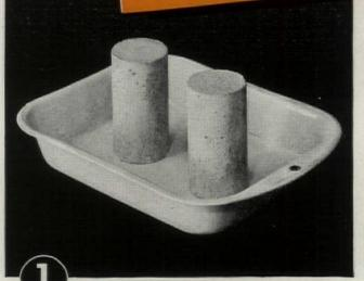
The photograph above shows a cylinder of Brixment mortar (left) and a cylinder of mortar made with portland cement and lime (right). Both specimens were made at the same time, and subjected to exactly the same treatment. After curing for 30 days, 1/4" of water was put into the tray and the
