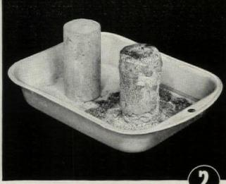
cylinders were alternately frozen and thawed 15 times. Note in photo 2 that the Brixment mortar remains intact, whereas the other mortar has crumbled badly. This simple test can be made in any ice-manufacturing plant, or in the freezing unit of a domestic mechanical refrigerator.
