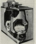
Both of these units are built around the Timken Model H wall-flame oil burner, which has only one movable part, and this part is self-lubricating by a forced feed system. The burner is equipped with the patented Timken chromium steel flame rim, which is said to cut warm-up time 87%. Leads for the electric ignition are of equal length and
