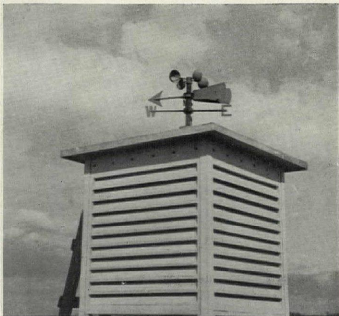
THE CHOATE SCHOOL SCIENCE CURRICULUM INCLUDES METEOROLOGICAL STUDIES, HENCE THE LOUVERED STRUCTURE ON THE "CAPTAIN'S WALK" ATOP THE SCIENCE BUILDING IS OF MORE THAN USUAL IMPORTANCE AS IT HOUSES SOME OF THE SCIENTIFIC DEVICES CONNECTED WITH INSTRUMENTS IN THE LABORATORIES ON FLOORS BELOW. NOTE DETAIL PHOTOGRAPH (BELOW) MADE BY T. JEBB AND T. TYLER
