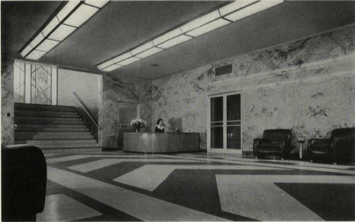
These two views of the Lobby show the marble floor and walls, and acoustical tile ceilings which add to the dignity of the entrance. In the background (above) may be seen the main stairway leading to upper floors. More than 100,000 watts of fluorescent light produce an average of 40 to 50 foot candles of light intensity throughout the building
