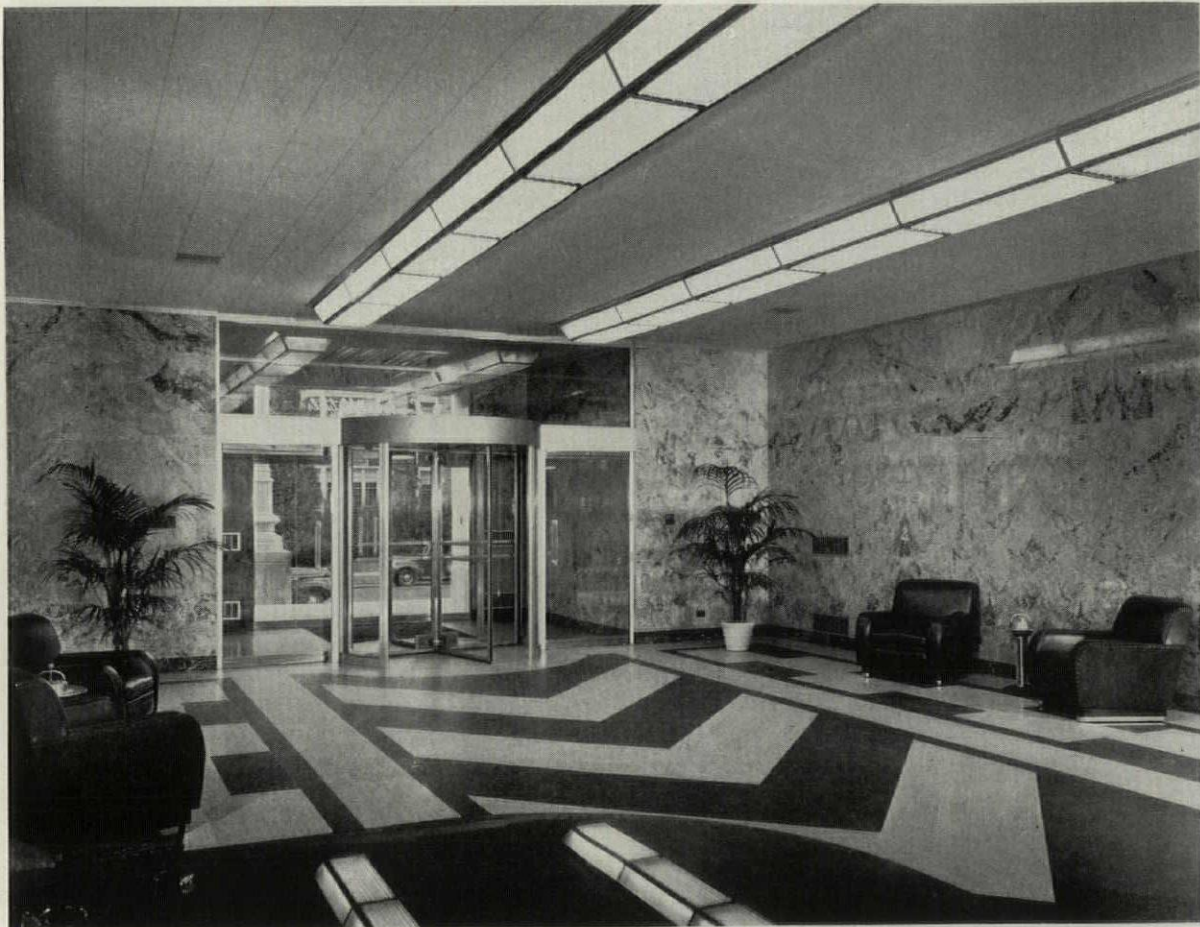
These two views of the Lobby show the marble floor and walls, and acoustical tile ceilings which add to the dignity of the entrance. In the background (above) may be seen the main stairway leading to upper floors. More than 100,000 watts of fluorescent light produce an average of 40 to 50 foot candles of light intensity throughout the building
