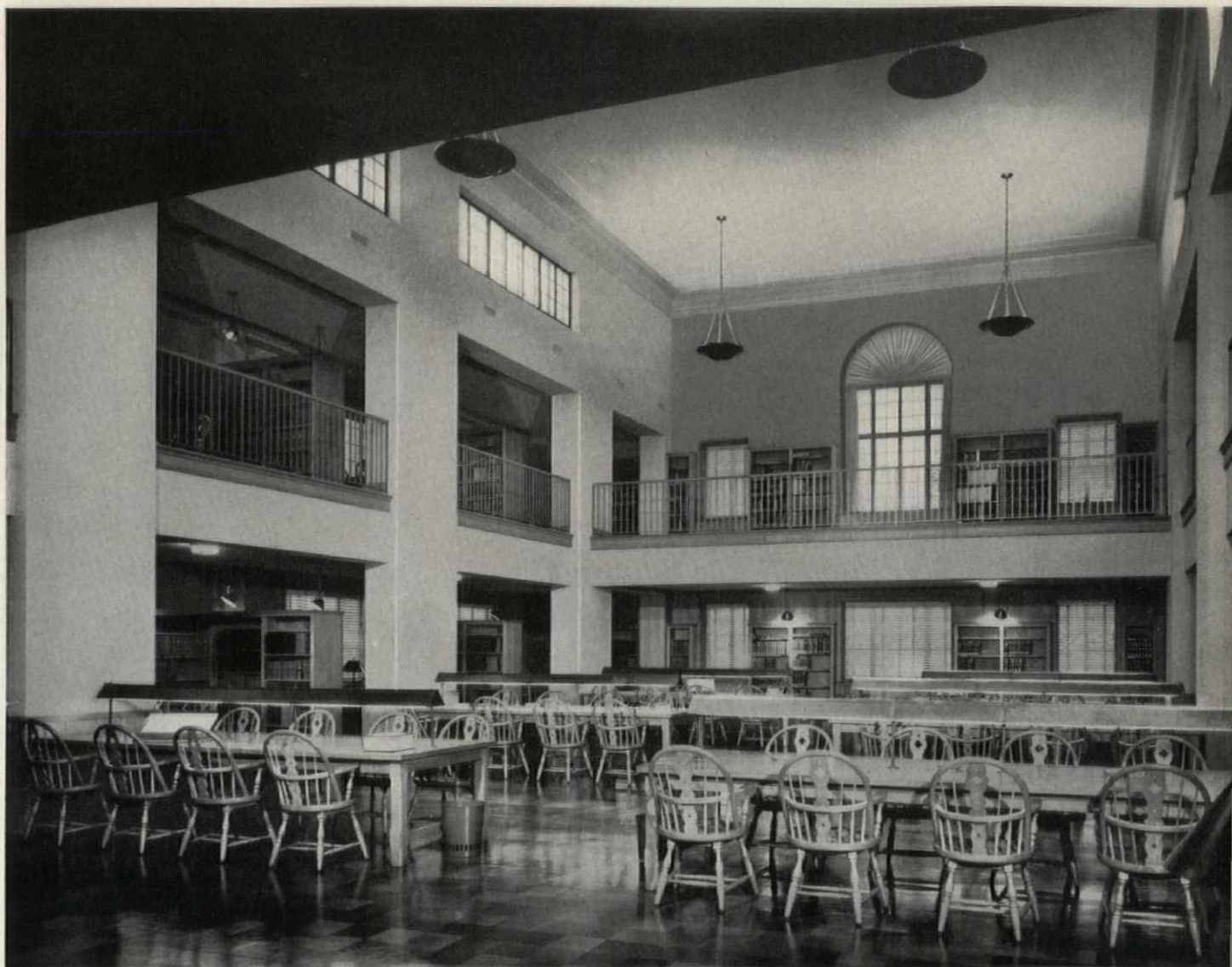
The General Medical Library (above) is strictly utilitarian, with cork tile floor and acoustical ceiling. The bottom shelf of every stack is set in at an angle so that the books tilt inward and titles are easily read by one standing before the case. Construction of building is brick and limestone on steel frame
