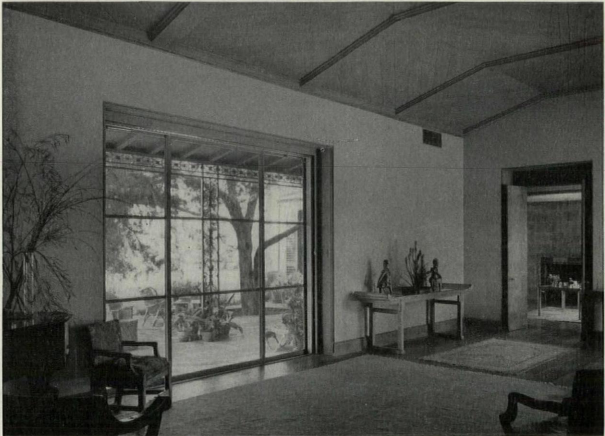
Opposite the fireplace in the Living Room, this broad opening frames a view of the lake. The warm color of the redwood ceiling shows through a semi-opaque parchment finish. The Morning Room (below) has hand-blocked wallpaper and a ceiling of bright metal-leaf
