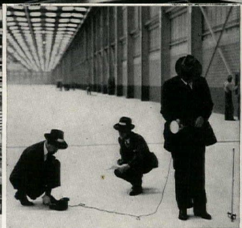
● White cement floor saves lighting and air-conditioning facilities and thus conserves rubber, metals, and power. Over 300 light measurements (see small picture) show white cement floor had 60% higher reflection factor than gray floor in same plant and increased vertical illumination 20%.
