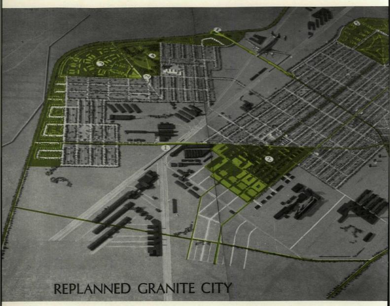
A survey of existing traffic conditions was first made, including points of congestion and danger, sources of traffic, destination of traffic, and traffic flow over main streets. The problem was then studied for redistribution of traffic flow, relief of congestion, and safe driving conditions.
