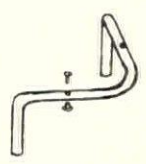
1 1/2" ROUND BENT OAK LEGS - SCREWED TO FRAME
