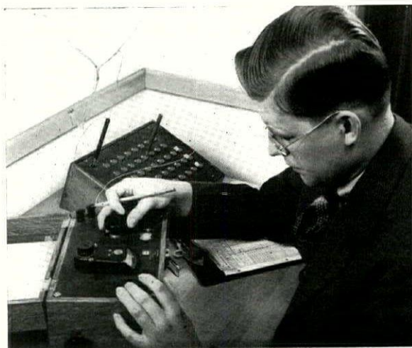
At night, temperature readings being taken with potentiometer at central panel.
