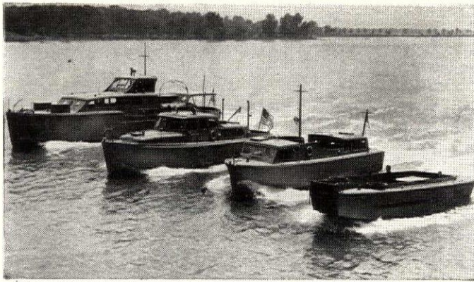
Four outstanding boats built by Chris-Craft with exterior-type fir plywood: (from left) U. S. Army Q boat, U. S. Army Aircraft Rescue boat, U. S. Navy Picket boat, U. S. Navy Troop Landing boat.
