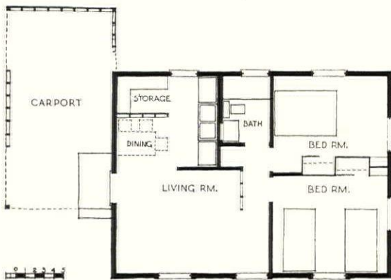
Plan of a typical "egg-crate" house; photos show a building whose plan was reversed. Platform at living room door is changed or omitted as site conditions demand.
