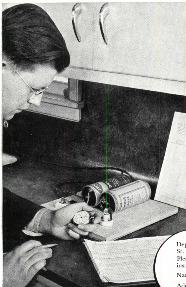
Checking wind velocity by timing period between flashes of lamp activated by electric cup anemometer.
