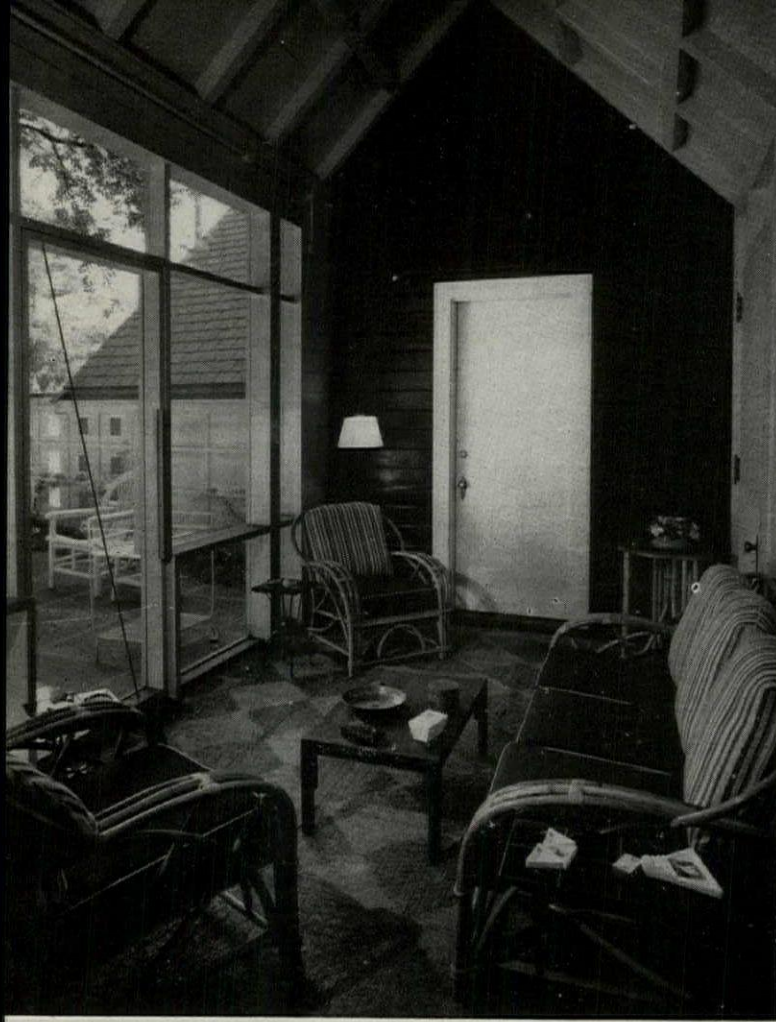
Living porch, showing use of discarded 4" x 4" shoring for framing members
