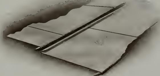
FIG. B.—FLAT-SEAM TIN ROOFING
