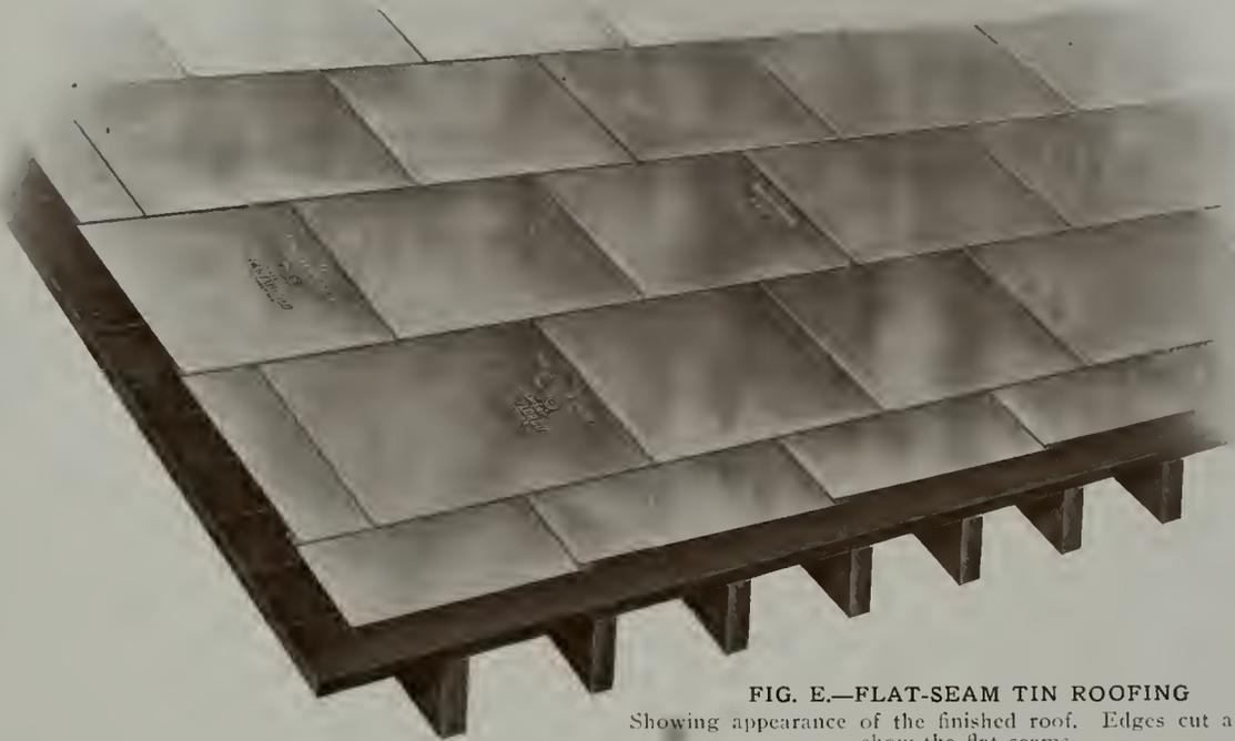
**FIG. E.—FLAT-SEAM TIN ROOFING**
