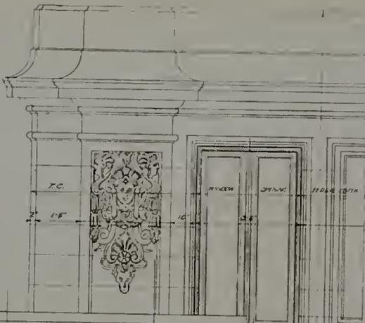
SCALE ELEVATION TYPICAL FOR PANELS OVER COUPLED COLUMNS AND PILASTERS
