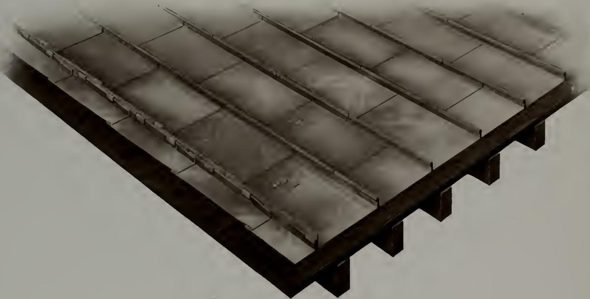
FIG. K.—STANDING-SEAM TIN ROOFING
