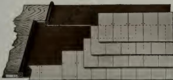
This is the usual square butt shingle (No. 16) commonly employed in laying either natural slates or Asbestos "Century" Shingles by the "American" method.
