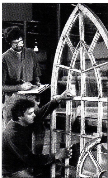
Workers from ADAMS ARCHITECTURAL WOOD PRODUCTS take precise measurements to ensure that the reproduction window will match the original. Write in No. 1265
