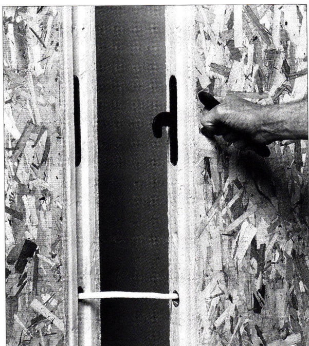
The MURUS structural insulating panel shown here is made from OSB/polyurethane/OSB, and can be joined with a patented cam-lock connector.
