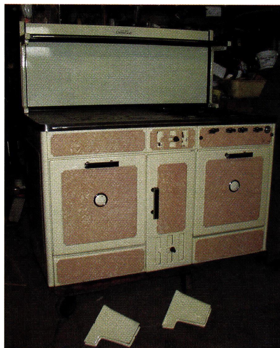
Left: This Gold Medal Glenwood range was purchased by Emery Pineo, president of the Antique Stove Hospital, from the daughter of the man who actually built it in the early 1930s. “We have restored it with new wood grate/liner, rebuilt the gas side and installed electronic ignition so that we could save the broiler,” he says. “Usually, the broiler cannot be saved if we use standing pilots in the oven.” Photo: courtesy of the Antique Stove Hospital
