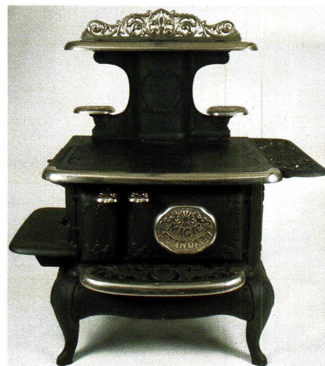
Left: This Gold Medal Glenwood range was purchased by Emery Pineo, president of the Antique Stove Hospital, from the daughter of the man who actually built it in the early 1930s. “We have restored it with new wood grate/liner, rebuilt the gas side and installed electronic ignition so that we could save the broiler,” he says. “Usually, the broiler cannot be saved if we use standing pilots in the oven.” Photo: courtesy of the Antique Stove Hospital
