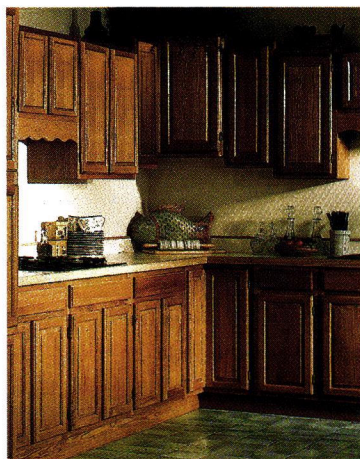
Most of Outwater's kitchen cabinetry features solid-plywood box construction with solid-oak or birch face frames, doors and drawer fronts.
