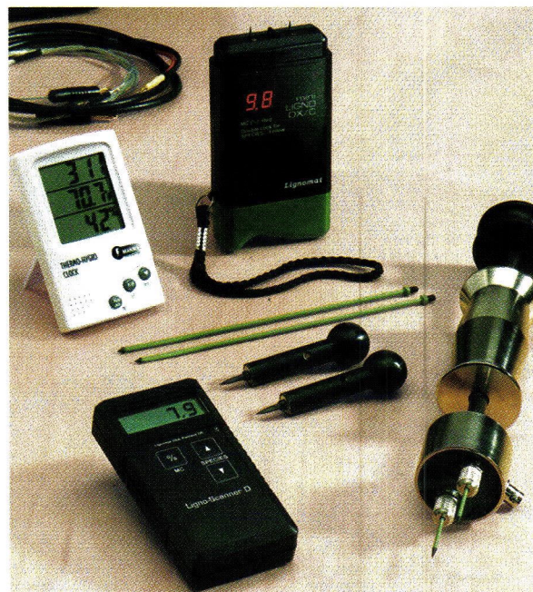
Lignomat manufactures hand-held moisture meters and thermohygrometers.
