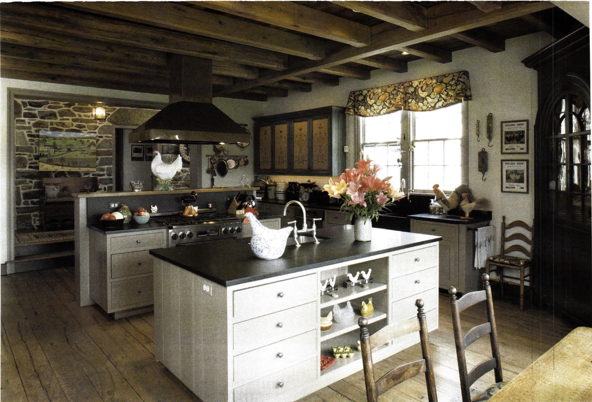
In the new kitchen, random-width oak flooring and oak ceiling beams were sawn from salvaged antique barn timbers. The exposed stonework represents the rear façade of the original 1800 house.
