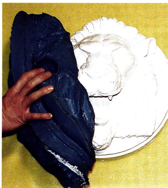
MasterMold, a non-toxic polyurethane paste from Abatron, is used to reproduce both large and small flexible molds.
