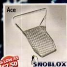
Face: 5" W x 3" H Base: 3" W x 5" L Waffled base increases bonding power. "V" shape fits most panels and does not trap water. Adhesive tested: 1449 lbs. SNOBLOX Screw tested: 4849 lbs.
