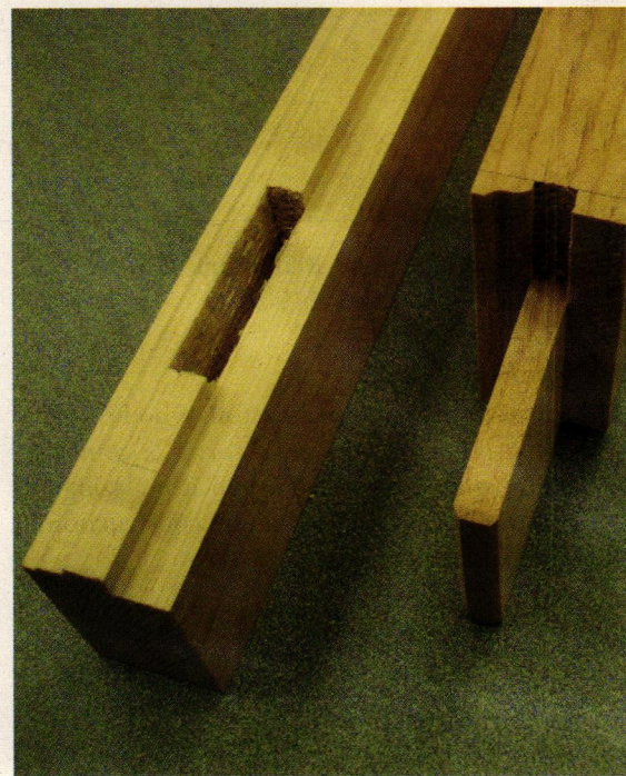
Weston Millwork uses mortise-and-tenon joinery for sash construction.
