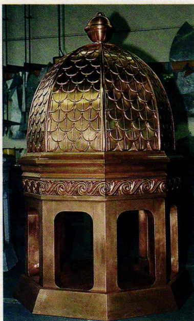
This copper-clad cupola, measuring approximately 10 ft. tall, was custom fabricated by Hans Liebscher for a residence in Nevada.
