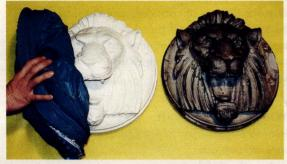
MasterMold, a non-toxic polyurethane paste from Abatron is used to reproduce both large and small flexible molds.
