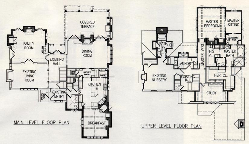
The firm expanded the kitchen by relocating the breakfast area to a new addition on the front elevation; an existing covered porch was replaced with a family room and the dining room was widened by extending the south wall. The upper level includes a new bathroom and master suite. Floor plans: courtesy of Harrison Design Associates
