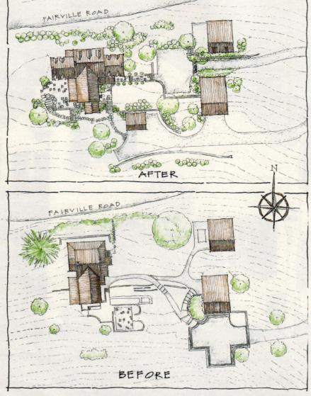
Before the renovation, the driveway terminated behind the existing stone barn and the original three structures were connected by a series of walkways; post-renovation, the new formal driveway creates an entrance courtyard between the four structures. Site plan: courtesy of Peter Zimmerman Architects
