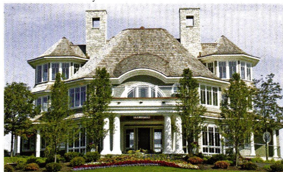
A Cedar Shake & Shingle Bureau member provided the cedar roofing for this house; the shakes are lightweight and have a high insulation value.
