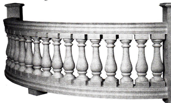
HB&G manufactures curved balustrade systems in 10-ft. sections by molding high-density urethane around structural elements.
