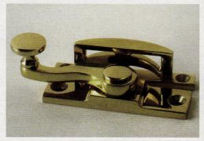
The model LK381 sash lock from Phelps Company features a patented design that draws sash together tightly while aligning them vertically; it is made of hot-forged solid brass and is hand polished.
