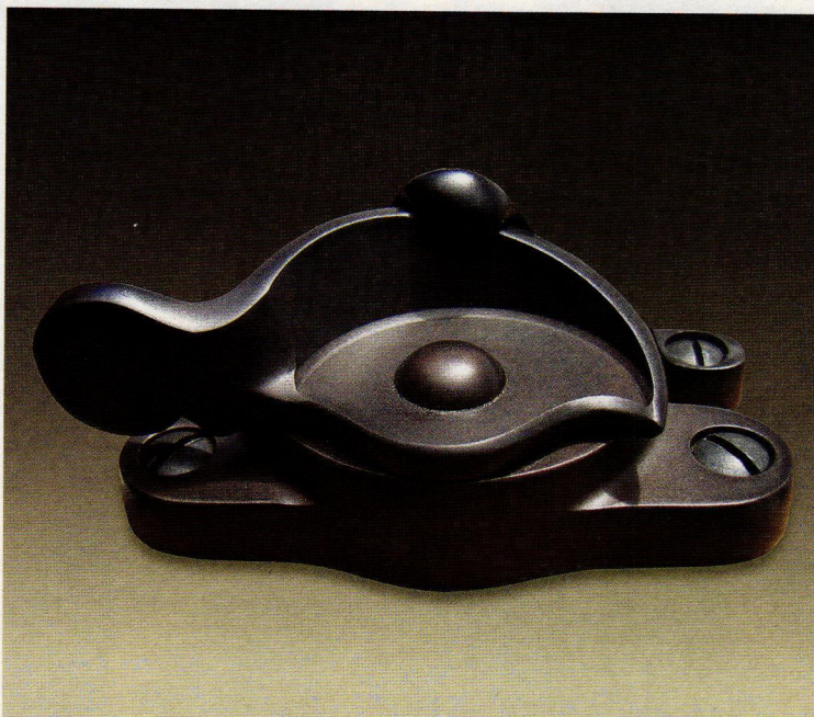
The model LKF18 sash lock from Phelps Company is hot-forged from solid brass and CNC machined; it features a double stainless steel spring mechanism for smooth operation. Click on No. 6001
