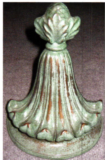
Triple-S Chemical's Green Verde #444 New was used to give this element its patina.
