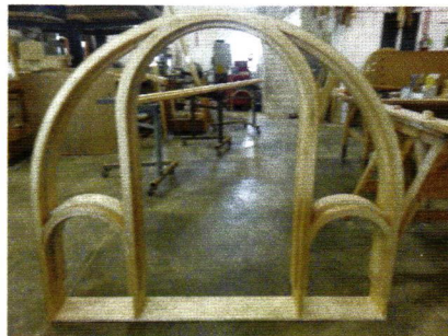
Arched Casings, Inc. , created this window using their CNC router
