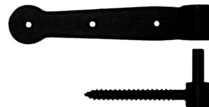
The traditionally styled mini strap hinge from John Wright Co. is made of 1/4-in.-thick cast iron; it measures 6 1/4 in. x 1.1 in. and provides a 3/8 in. offset.
