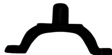
This porch post iron from John Wright Company secures a post while providing a standoff to prevent the bottom of the post from rotting; it works with most 4- and 5-in. posts.
