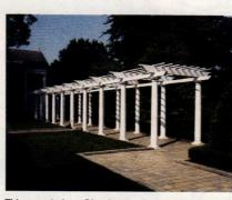
This pergola from **Chadsworth** was fabricated from cellular-PVC beams and rafters and PolyStone support columns. Click on no. 1580.
