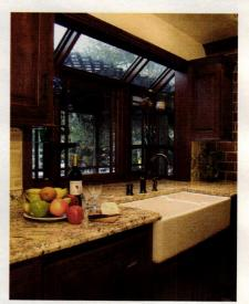
Renaissance Consservatories manufactured this custom garden window in solid mahogany; the hardwood specie, finish, grids and exterior roof cladding are all customizable and can match interior millwork and cabinetry.
