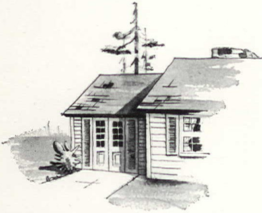
How to eliminate a big garage door: French "door" and adjoining panels fold back to admit the car
