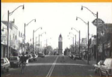
Above: On Welch Avenue, in Ames, Iowa, street lights were placed in the parking lane as an alternative to trees for establishing vertical definition. Right: Castro Street in Mountain View. The street was reduced from four traffic lanes to three, and the extra space was used to create wide, flexible-use “overlap zones” on both sides.
