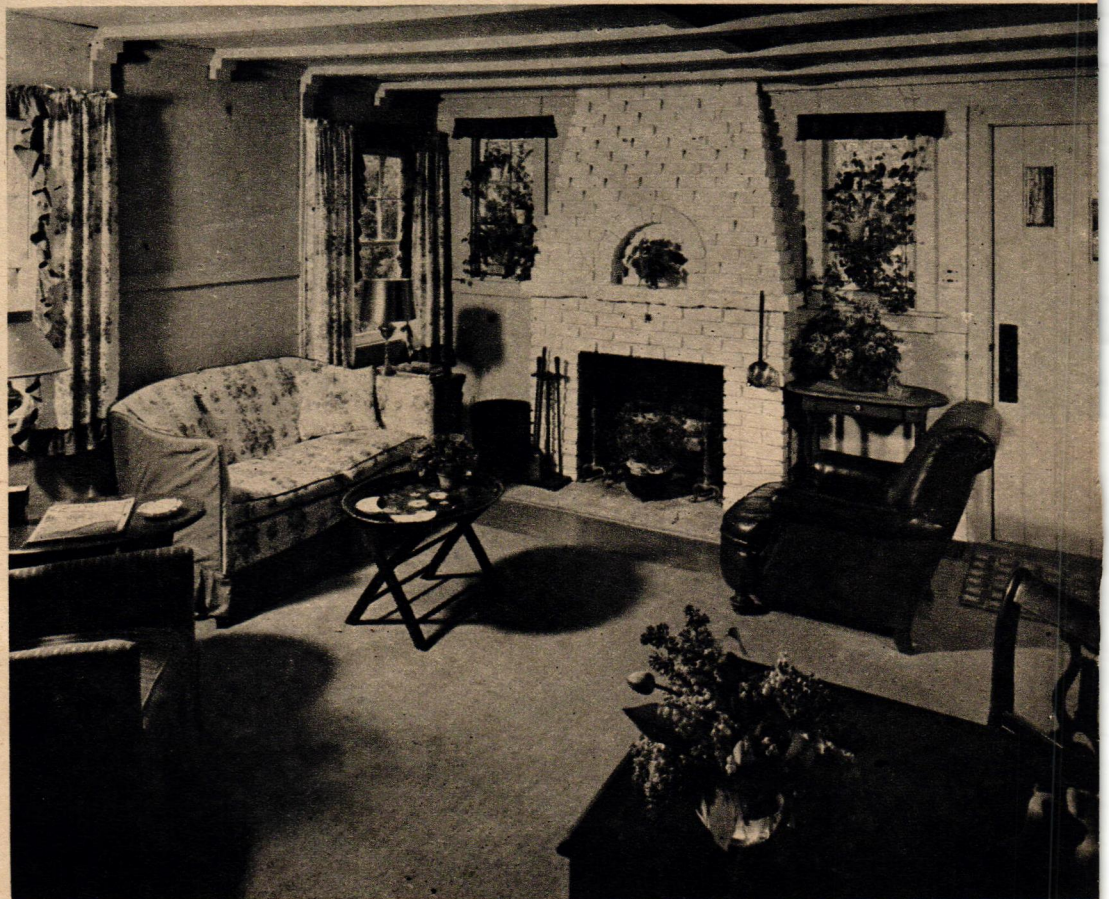
This was not a job for unlimited expenditure. The fireplace was retained unchanged, and most windows were left intact. SHEETROCK wallboard had its joints covered with batten strips and was painted with TEXTONE, a texture paint in smoke grey.
