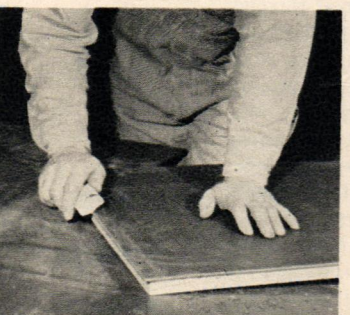
8 Start rounding the lip edges with a plane. Then sandpaper edge to smooth, uniform curvature.
