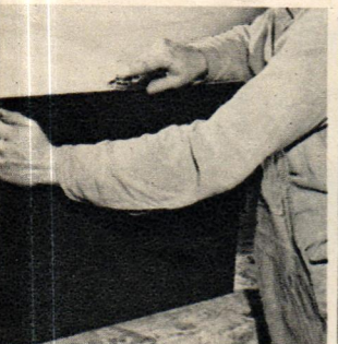
7 If a back panel is used, put it on before the front panel. Plane edges flush with frame.
