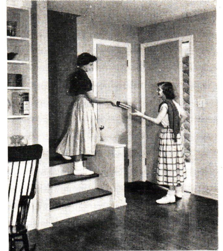
Out-of-style doors are easy to convert to flush doors. Remove glass, fit large glass openings with cross pieces for strength, face with DURON hardboard, trim edges, and paint. Doors now look new (right).
