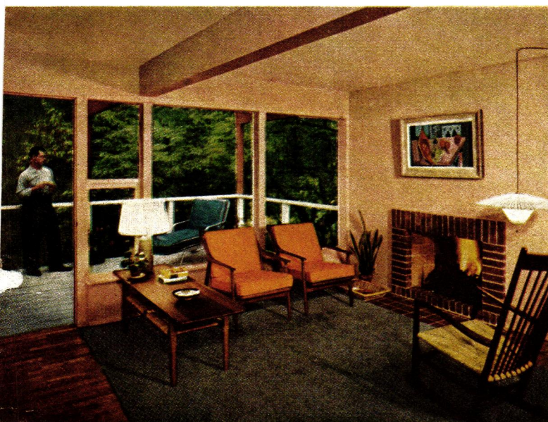
To accent view outside, ceiling and only wall adjacent to windows are smooth (standard SHEETROCK gypsum wallboard with joints concealed by PERF-A-TAPE joint system). Warm, muted colors like TEXOLITE DURAVAL paint's Russet Beige also complement view of garden and foliage outside.
