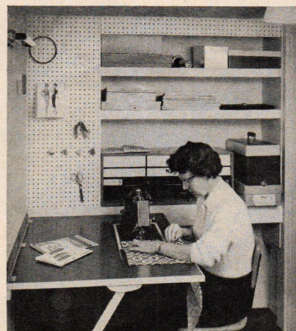
Ideal sewing center is easy to build. Shelves are 1x10's with 1x2-in. edging. Perforated hardboard hides piping, provides handy storage space for much-used items. Cutting and sewing table, made of ½-in. plywood, hardboard and doorstop molding, folds out of way.
