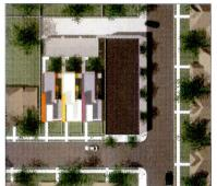
A 10-foot recess in the front, south-facing elevation keeps direct sunlight out of living areas, except in winter, and the facades have commercial-grade, operable windows. The townhouses touch a commercial building that Sprinkle Robey renovated (left). Amenities include a detached two-car garage, concrete floors, and, in front, a 20-foot square of lawn. The architects envision a stand of bamboo behind the wall for screening.
