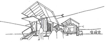
The extendable parasol roof accommodates solar tiles and shields the structure from the sun. Folding sleeping platforms and tables keep interior spaces simple and utilitarian.
