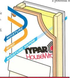
Typar is proven to offer the best combination of keeping water out and allowing moisture vapor to escape from the wall cavity.
