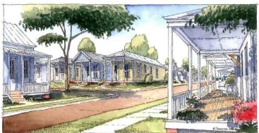
Conceived as an alternative to trailer- and mobile home—based transitional housing, the Mississippi Cottage is a temporary dwelling that can become a permanent home (top and right). Built like a modular home but delivered on a wheeled chassis, it comes in two- and three-bedroom versions. Its Gulf Coast vernacular design has made it the basis for a number of successful permanent neighborhoods (above).
