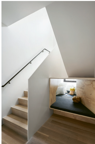
A plywood-constructed portal leads to a sitting area behind the staircase, made sculptural with white-painted steel plates welded together.
