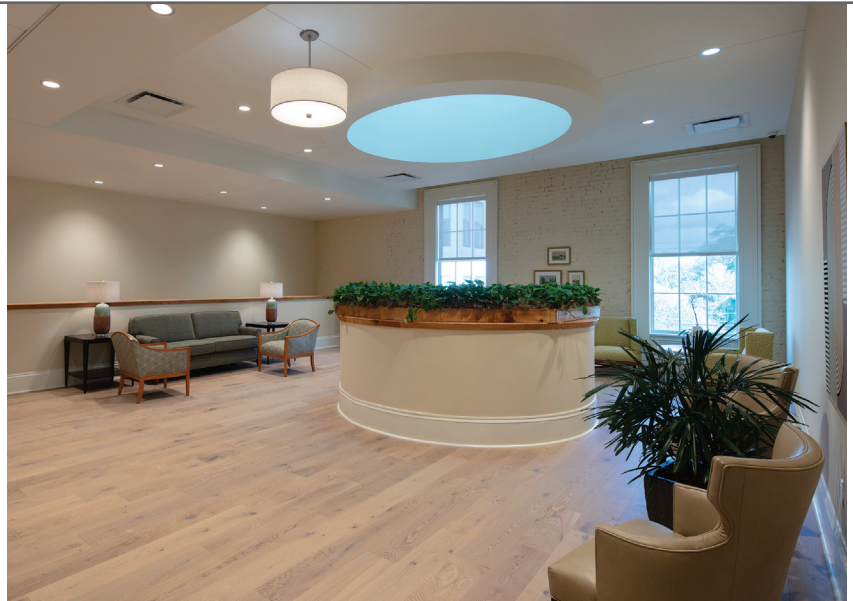
Reclaimed wood framing from the historic structure was milled and repurposed into a custom entry desk and a rail cap in the light well.
