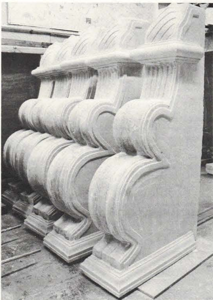
Brackets (with styrofoam cores) were precast in architectural concrete by ARCHICAST as part of the reconstruction of an Italianate cornice.
