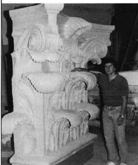
"After casting 10 large fiber-glass parts, the mold was in such good condition we could have made 50 more." The 8 ft. by 7 ft. corinthian column capitals have 24 inch undercuts.
