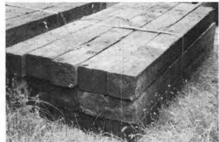
These #1 grade used railroad ties are mainly used in landscaping for retaining walls. The dimensions are: 7 X 9 X 8-1/2 inches, and they are available from MIDWEST RAILROAD TIE SALES.
